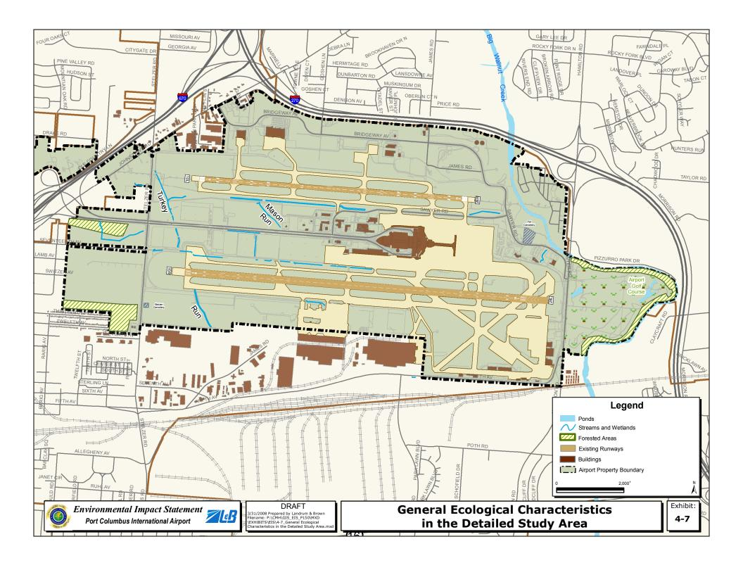
The drainage network discharging to the lower reach of Mason Run originates on the south side of Runway 10L/28R. Mason Run flows southeast under International Gateway to a series of box culverts passing under Runway 10R/28L and under former Air Force Plant 85 (currently Million Air, Inc. and the Columbus International Air Center (CIAC)). Mason Run is enclosed for approximately 2,000 feet under former Air Force Plant 85.<sup>10</sup>
